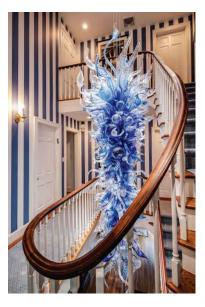
In a 2nd HOBI win, Gatehouse used a steel mounting plate, reinforced rafters and cables rods to achieve a striking interior home feature with this one-of-akind hand blown glass light fixture that weighs one ton.
